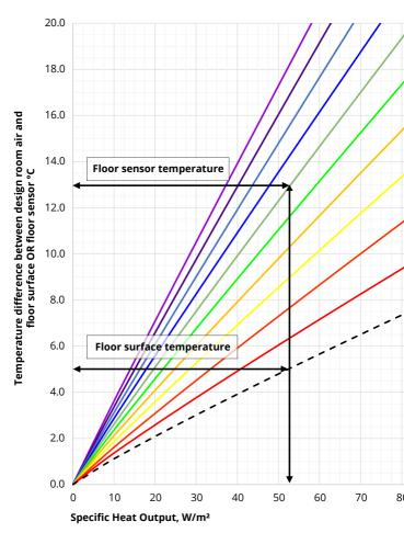
Using the graph above it is possible to get the specific heat output of an electric underfloor heating system based on the temperature difference between the design room air temperature and the floor surface or floor sensor temperature by floor finish.
