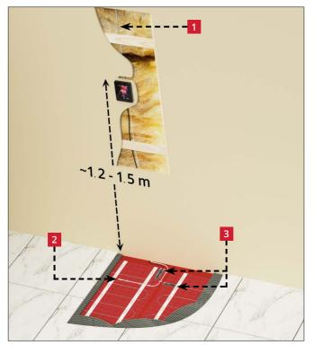
The supply to the thermostat MUST be protected by a 30mA RCD or RCBO at all times. Time delay RCD's or RCBO's must not be used. No more than 7.5 kW of heating should be connected to each 30 milliamp RCD or RCBO. For larger loads, use multiple RCD's or RCBO's.
